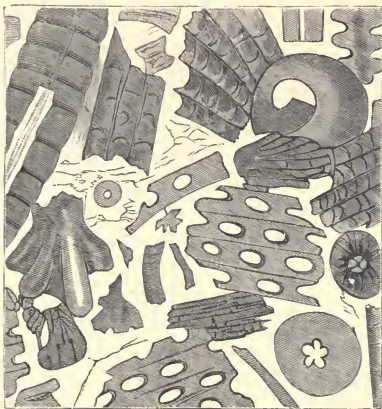
Fig. 9.—Fragment of Lower Silurian Limestone, sliced and magnified ten diameters, showing the manner in which it is made up of fragments of corals, crinoids, and shells. (From a paper on the Microscopic Structure of Canadian limestone, "Canadian Naturalist.")
